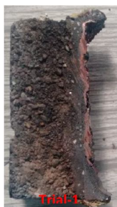
Figure 2: DBMC brick after the test
