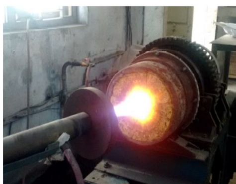
Figure 1: Furnace for standardized slag Corrosion tests
